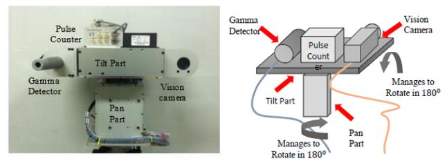
Figure 1: Experiment setup at a glance.
