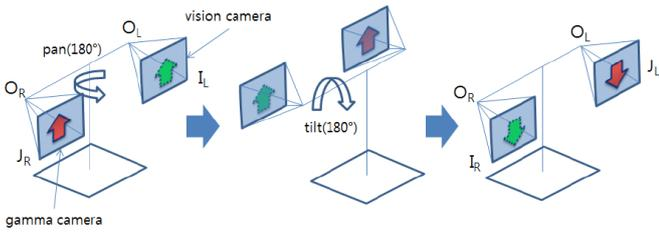
Figure 2: Panning and tilting of the setup to obtain stereo gamma and vision images.
