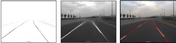
Figure 7. Result of the curved lane detection
