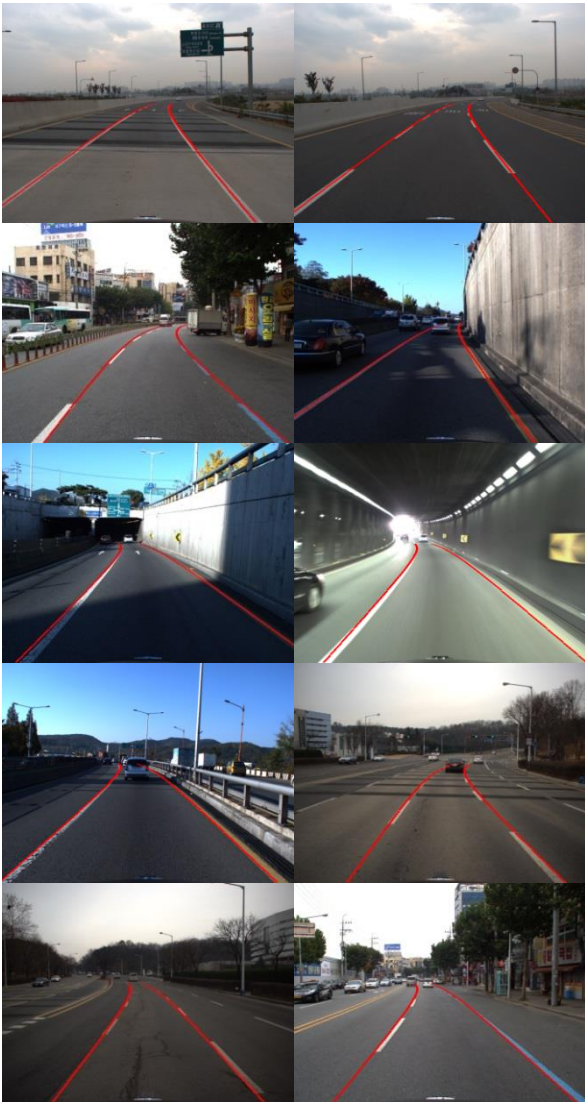
Figure 9. Result of the curved lane detection.
